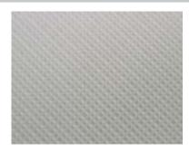
Medium (30%) - The selection gives higher strength to the structure than low density. To print an object for mechanical purpose, it is advised to set the density to 30% or above.
