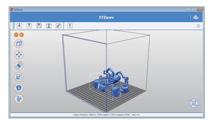
By default, all .stl files will be printed from extruder 1. You may assign one object to be printed from extruder 2.
