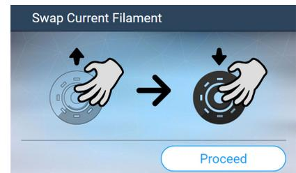
5. The nozzle will be preheated and the machine will notify you when to insert filament into the feed module.
