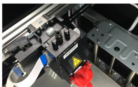
7. Press the white release button to separate the print head.
