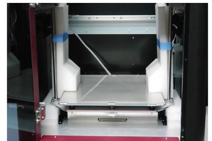
**9** Remove the cable tie and foam situated behind the front door.
