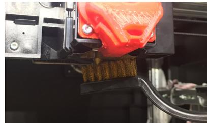
3 Use the tweezers to hold the extruder cleaning wire, and insert the wire from the bottom of the extruder to clear the extruder opening.
