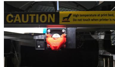
When the temperature of the print head reaches the operating temperature, the cleaning operation starts.
