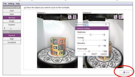
When the software starts generating the point cloud and 3D model, you can rotate, zoom in or zoom out using your mouse in the Preview pane to view the scan results.
